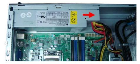
5. Tilt the power supply module slightly to the right and lift it out of the chassis.
